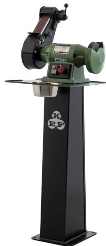
Special grinder for sharpening of knives, etc.
