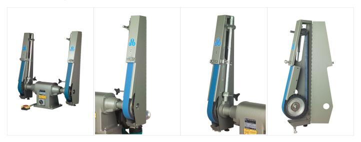
KEF professional heavy double industrial grinders BO is characterized by a simple but strong stable construction. The great distance between grinding arms makes these machines very suitable for grinding of curved issues. The machines are available with one and two speed and can be fitted with an abrasive band on one side and polishing belt on the other side. The BO machines have a low noise level both mechanical and electrical.
