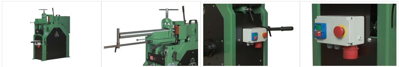
Pipe grinders for grinding of all kinds of pipes and profiles before welding.
