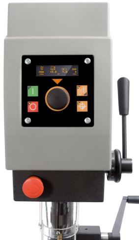
**MENU FEATURES** · Clear and understandable input menu · Mode selection between drilling and tapping · Two precise display values for target- and actual drilling depth as well as the speed · Counting function of drilling/threading strokes · Intelligent memory function of the set parameters · Automatic power saving mode.
